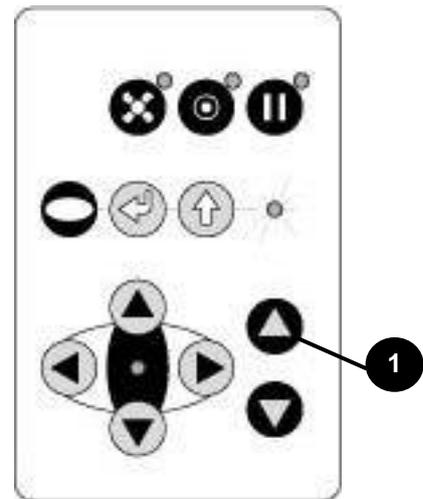
Before the focus tool reaches the work piece, move the working table upwards only very slowly and step by step by briefly tapping the positioning key, until the tool tilts to the side. Now the lens is focused onto the surface of the material.
