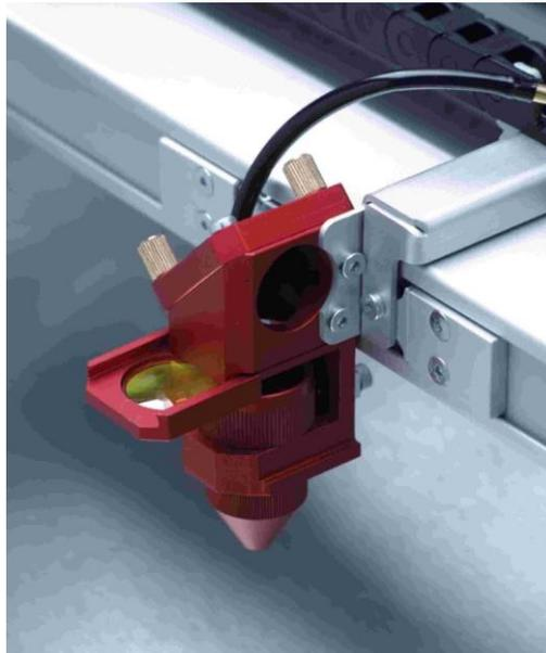
In the Trotec JobControl the lens must be selected under Settings>Options>Engraver or in the symbol bar "Laser Position" to make the autofocus work correctly.
