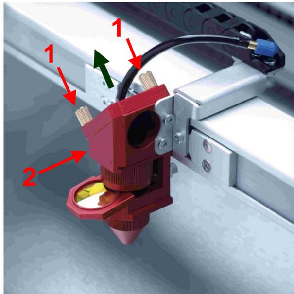
2. Use a drop of lens cleaning liquid from the accessories box and, while holding the mirror on an angle, flush the surface of the mirror, to wash away coarse soiling.
