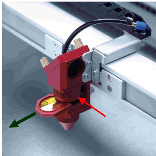
4. Remove the coarse dust as good as possible by blowing air onto the lens surface.
