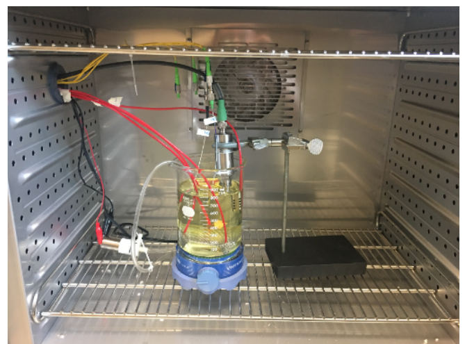
Sensors Testing in Humidity Chamber with Mineral Oil
